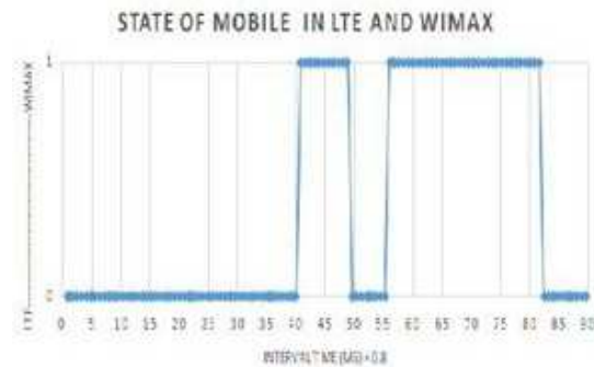
Fig. 4: State of Mobile node in LTE and WiMax for a time interval of 0.8 ms.
