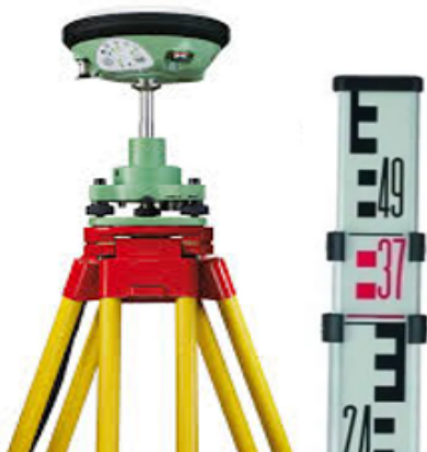
Fig. 3: LEICA VIVA GS14 GNSS used in the conducted research.
