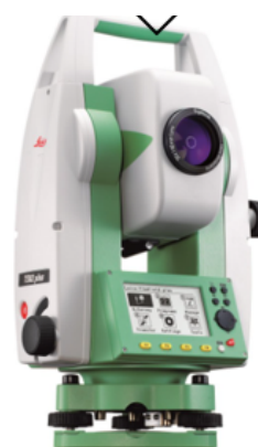
Fig. 2 : LEICA FLEXLIN TS02 PLUS TOTAL STATION used in the conducted research.
