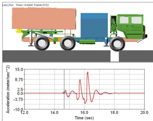
Fig. 12: Virtual test of low speed across trench
