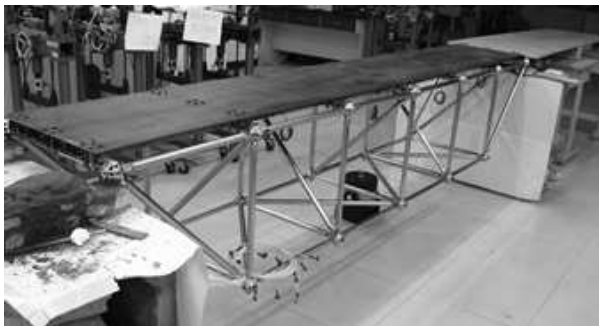
Fig. 1 Deck-truss bridge structure
