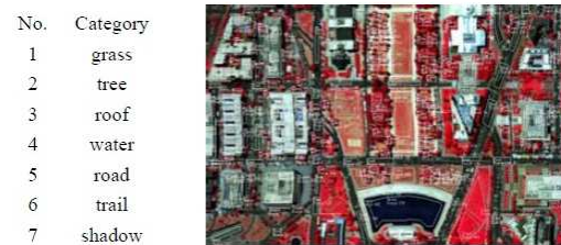
Fig. 4: The false-color IR image of a portion of Washington, D.C. Mall image with a size of 205x307 pixels. There are seven categories, grass, tree, roof, water, road, trail, and shadow.
