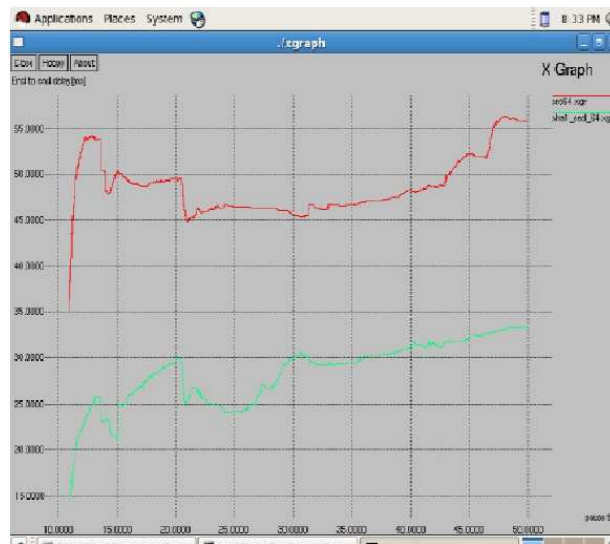
Fig. 4: End to End delay of CRC-32 and SHA-1 at 64 bit key
