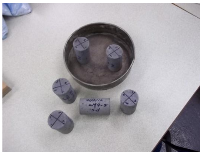
Fig. 3 - Specimens demoulded and ready for testing
