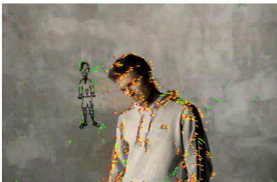
Fig.2 Optical flow segmentation example. (red dot: foreground, green dot: background, yellow arrow: optical flow)
