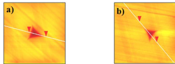
Figure 3: Atomic force microscopic images of indentations created in the surfaces of samples: (a) Sample c 2 and (b) sample c 5 .
