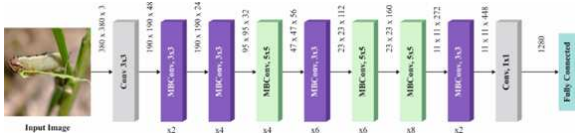
Fig. 2: Architecture of EfficientNet-B4 model
