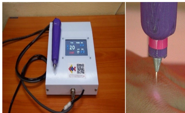
Fig. 1: (left) Air plasma jet production system (right) Air plasma jet
