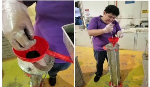
Fig. 8: Fill CR in the mold (before the Isocyanate).
