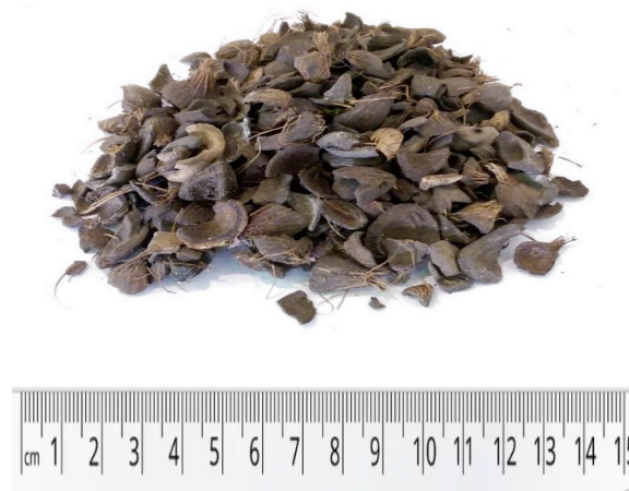
Fig. 1: ops Lightweight Aggregates (8 – 10 mm Size)
