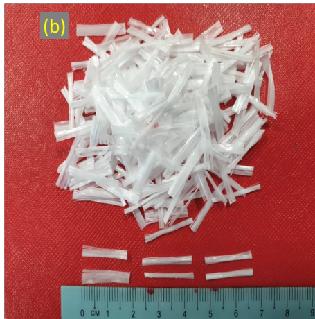
Fig. 2: Type of PP Reinforcement (a) PP Mesh Netting (35mm x 35mm x 2 mm diameter) and (b) Fibrillated PP fiber (19 mm length)
