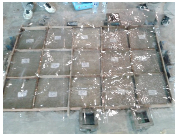
(a) Casting of slabs
