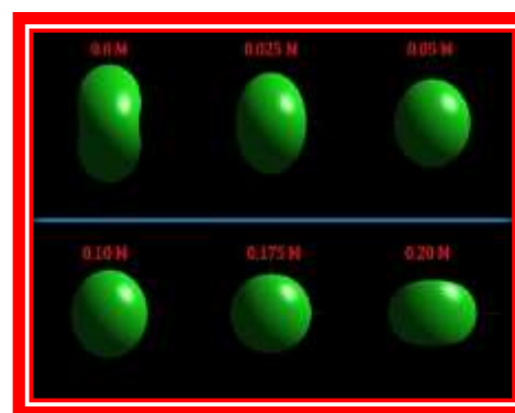
Fig. 4. Crystallite plot using Popa rules model for nanoparticles of ZnO synthesized at different concentrations of citric acid.
