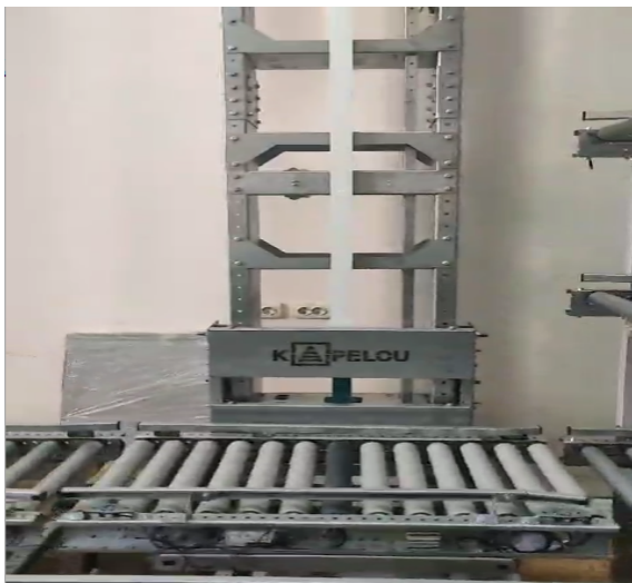
b) vertical industrial elevator for moving packages between floors
