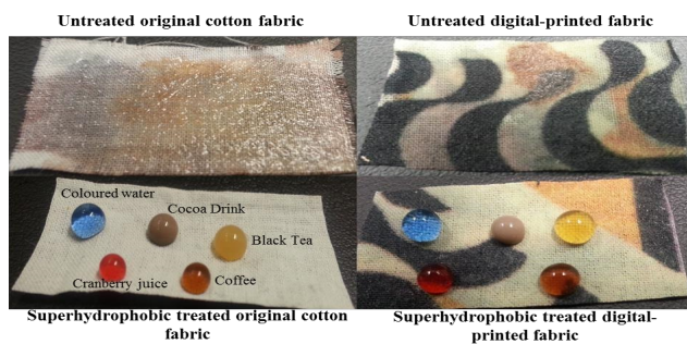
Fig.12. Images of various liquid droplets on the surfaces of untreated fabrics, and treated fabrics with coloured water, cocoa drink, black tea, cranberry juice and coffee.
