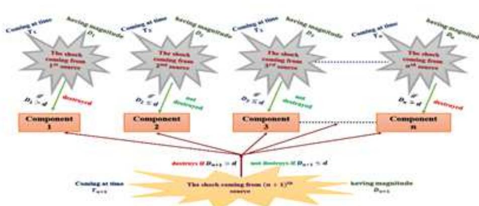
Fig. 1: A system with  $n$  components subjected to Marshall-Olkin type shocks concerning magnitude.
