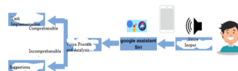
Fig.1: The implementation mechanism of voice command
