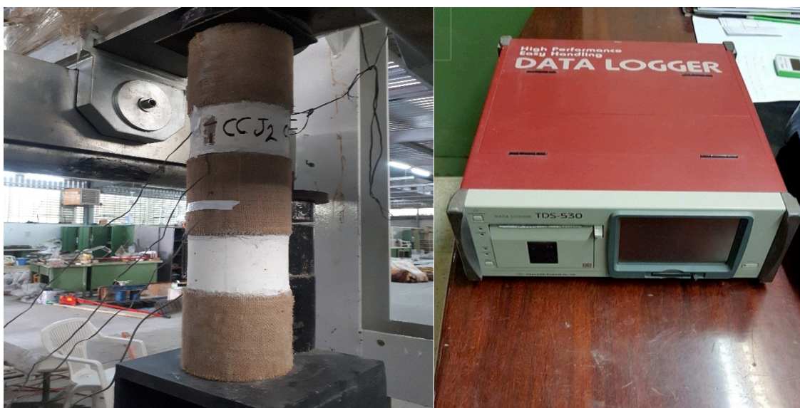
Figure 4: Data logger device and strain gauge installation
