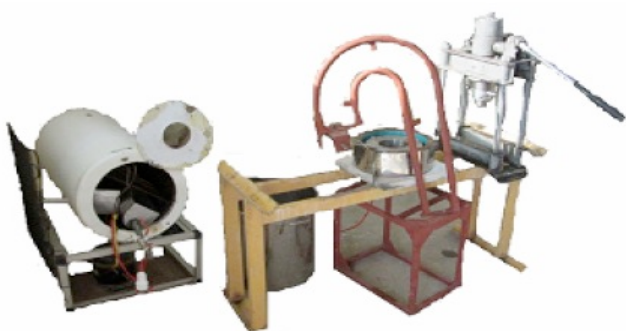
Fig.1: The recycling of marble and granite wastes unit.
