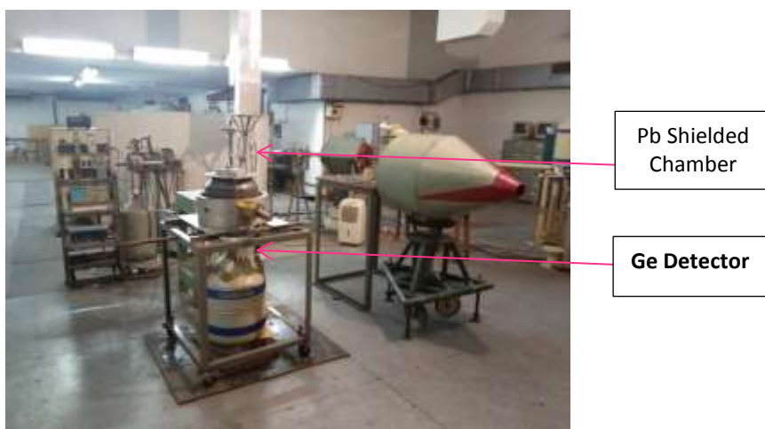
Fig.2: Photograph of ‘Lead Shielded Chamber with detector.’
