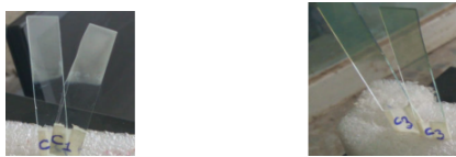
Fig. 2: Photo image of zinc sulfide thin film and copper zinc sulfide thin films on the substrate.
