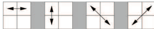
Fig. 5 Four directional neighborhood of a pixel (i.e. left to right, top to bottom, top-left to bottom-right, and top-right to bottom-left)
