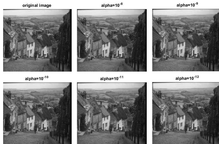
Fig. 5: Results of applying the proposed method on a dark image with different values of fractional parameter \alpha .
