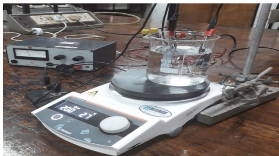
Figure 1. Experimental setup for anodization of the Zinc plates.
