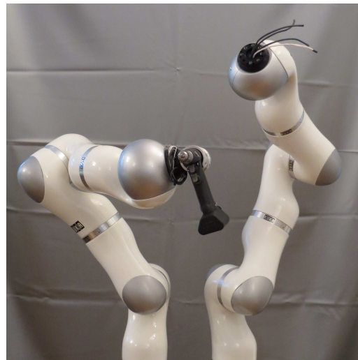
Fig. 1: The 7 degree of freedom KUKA LWR IV+ robot; this paper deals with one of the robotic arms only
