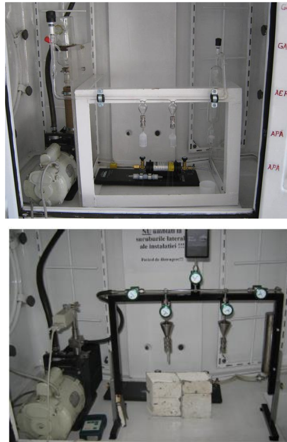
Fig.2: A glass and metallic circuits in Radionuclide Metrology Laboratory presents the 222 Rn Standard System.
