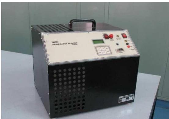
Fig.5: CRM based on electrostatic collection
