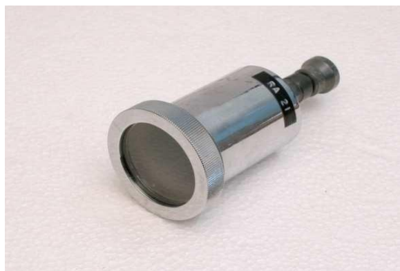
Fig.6: Lucas scintillation cell
