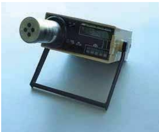
Fig.4: CRM using scintillation cell
