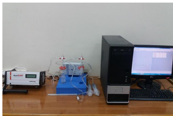
Fig.8: Detector Alpha GUARD (Genitron Instruments) in measurements of radon activity concentration in water.
