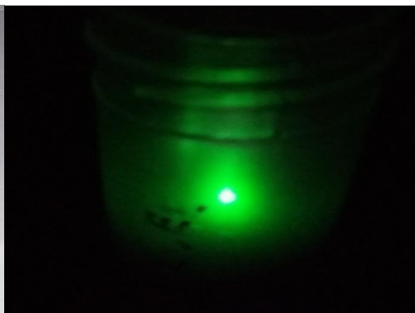
Figure 4.5 (b): Emission in green color upon excitation at 980 nm
