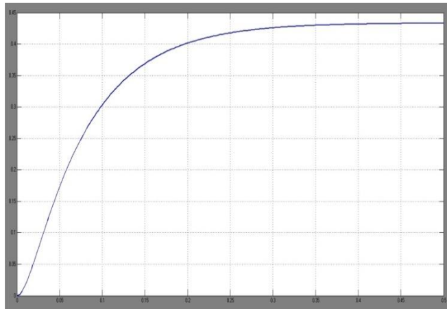
Fig.4. Step input of uncontrolled DC motor drive system.
