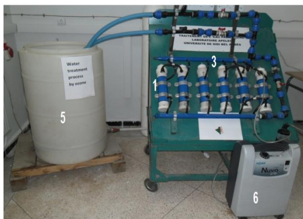
Figure 4: Photograph of the experimental setup (Front view) 1- Three ozone generators connected in series ; 2- Transformer High-voltage ; 3- Venturi injector ; 4- Water pump; 5- Water reservoir; 6- Oxygen concentrator.
