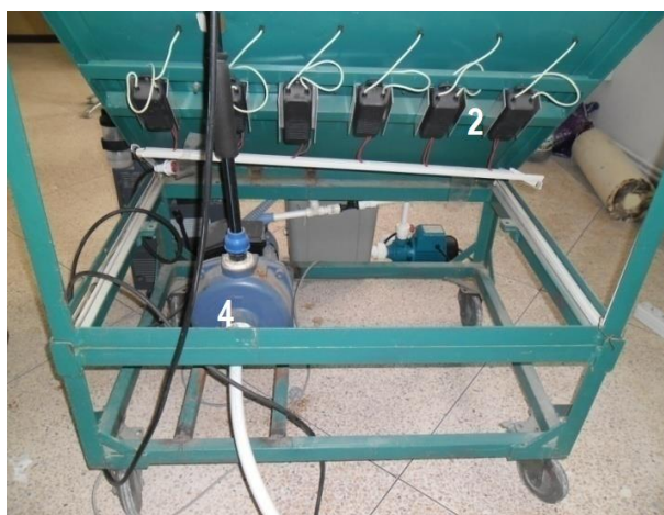
Figure 4: Photograph of the experimental setup (Front view) 1- Three ozone generators connected in series ; 2- Transformer High-voltage ; 3- Venturi injector ; 4- Water pump; 5- Water reservoir; 6- Oxygen concentrator.
