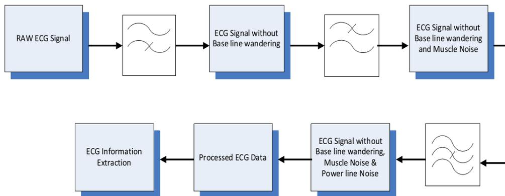
Figure 5. ECG Signal Processing Flow Diagram
