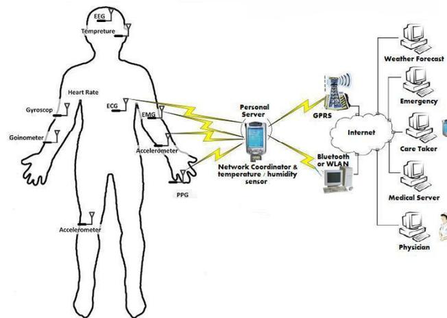
**Figure 1.** Wireless Body Area Network Scheme
