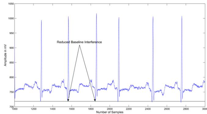
**Figure 15.** Blackman Harris Window based Highpass Filter
