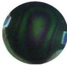
Figure 1: Photograph of 3C-SiC thin film deposited on thermally oxidized Si
