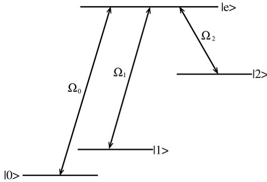
**Fig. 1:** Energy level for a four-level tripod. The three ground levels  $|0\rangle$ ,  $|1\rangle$  and  $|2\rangle$  are coupled to the excited level  $|e\rangle$  by three different lasers. The two ground states  $|0\rangle$  and  $|1\rangle$  are the states of the desired qubit.
