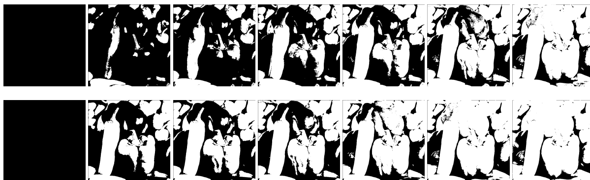
Fig. 2: the segmented images of pepper by UL-PCNN(the first row) and MUL-PCNN(the second row)
