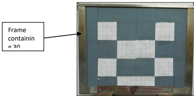
**Fig.1:** Arrangement of lead bricks.
