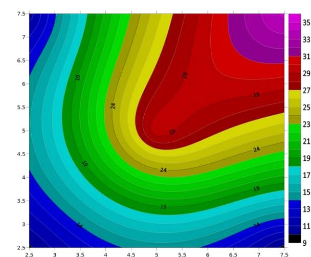
Fig. 10: Surface plot of gamma dose for specimen B2.
