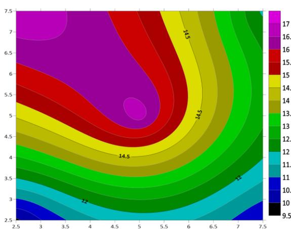
Fig.8: Surface plot of gamma dose for specimen C2.
