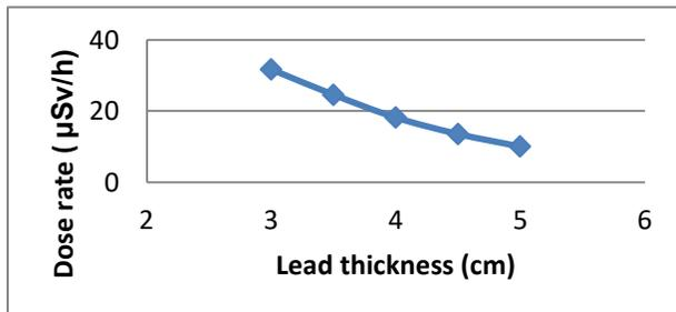
**Fig. 4:** Gamma transmission curve through defect free lead.
