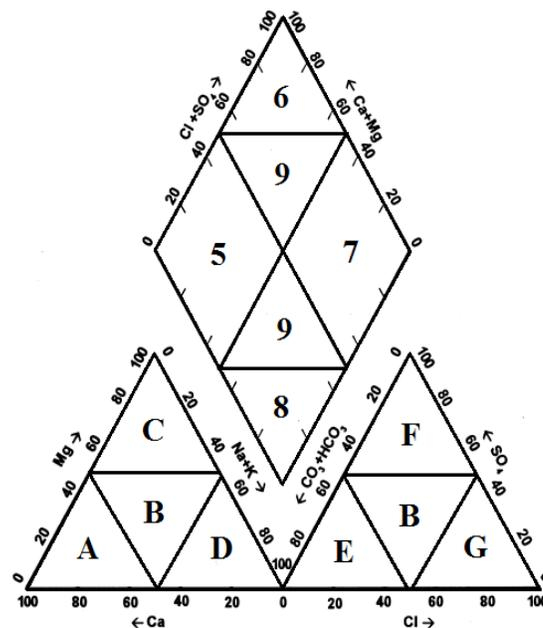
**Fig. 18 :** Piper's classification scheme.
