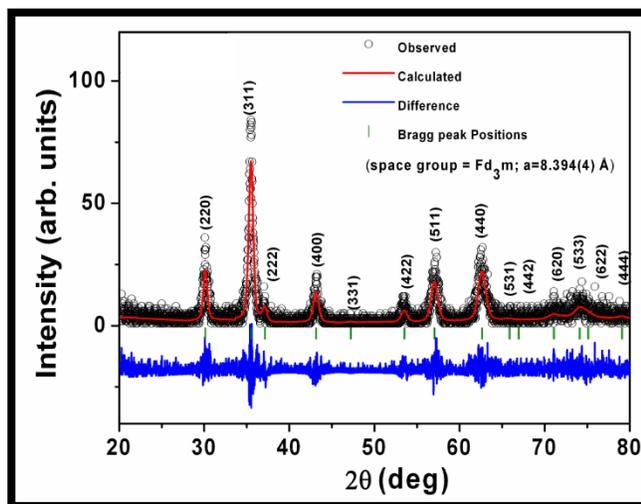
**Fig. 2:** Rietveld refined XRD patterns of gamma irradiated  $\text{Mn}_{0.7}\text{Zn}_{0.3}\text{Fe}_2\text{O}_4$  nano ferrites.
