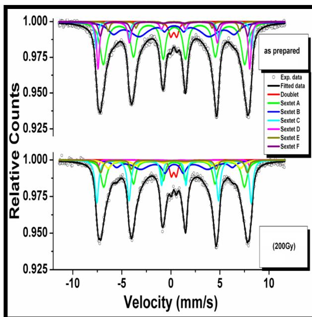
**Fig.3:** Mössbauer spectra of as prepared and gamma irradiated  $Mn_{0.7}Zn_{0.3}Fe_2O_4$  ferrite nanoparticles recorded at room temperature (300K).
