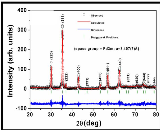
**Fig.1:** Rietveld analysis of as prepared  $\text{Mn}_{0.7}\text{Zn}_{0.3}\text{Fe}_2\text{O}_4$  sample.
