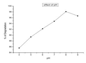
**Figure 5.** The Effect of pH on Adsorption at 25 <sup>o</sup>C and 100 mg Bentonite on 50 ml 200 ppm Malachite green Solution
