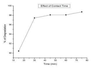
**Figure 6.** The Effect of Contact Time on Adsorption Rate on 50 ml 200 ppm Malachite green Solution with 100 mg Bentonite.
