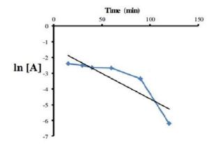
**Figure 9.** Kinetic Model of Pseudo- First Order for Bentonite on 50 ml Malachite green Solution
