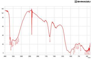
Fig. 2 IR Spectra of Bentonite Clay
