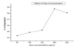
**Figure 8.** The Effect of Dye Concentration on Adsorption Rate at 25 <sup>o</sup>C on 100 mg Bentonite
