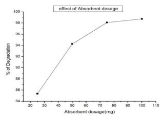
**Figure 7.** The Effect of Various Loading on Adsorption Rate with 50 ml 200 ppm Malachite green Solution
