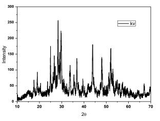
Fig. 3 X-Ray diffraction (XRD) of Bentonite clay
