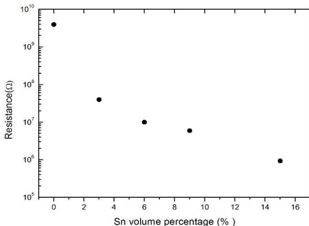
Fig.5. Resistance values of the CdS:Sn thin films.
